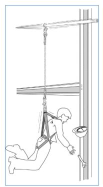
The attachment point (D-Ring) must be located in the center of the wearer's back near shoulder level.
