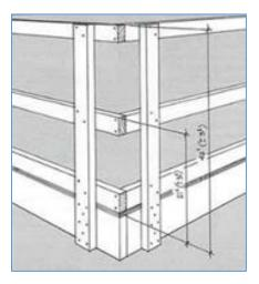
A guardrail must be strong enough to **withstand a force up to 200 pounds** applied to the top rail in an outward or downward direction.
